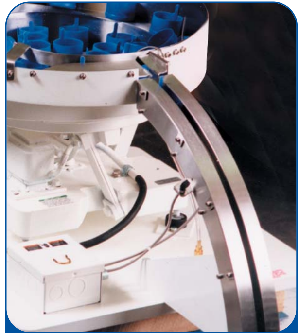
Syntron® Gravity Tracks send plastic parts to the next assembly stage.
