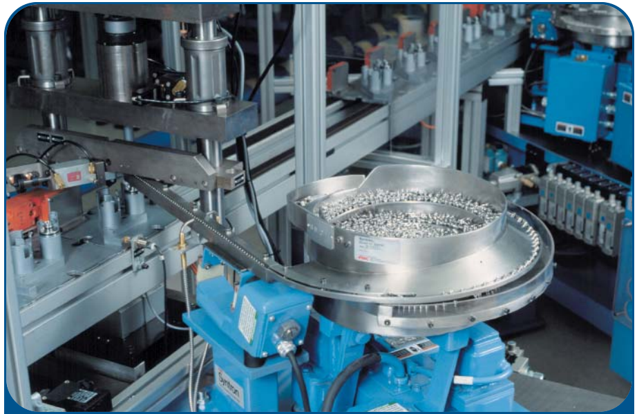
Syntron® outside track bowls are ideal for applications requiring intricate tooling to orient parts.
