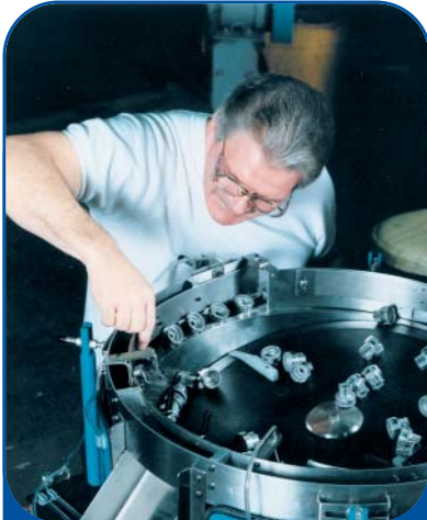
This rotary feeder, designed to singulate bolts, gets a final inspection from our quality control personnel.
