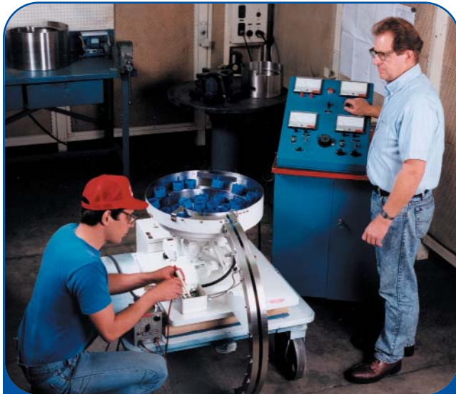
Once final adjustments are made, an electrical test is conducted to assure correct voltage and amperage for designated electrical standards.
