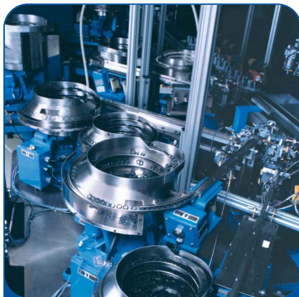
A group of Syntron vibratory parts feeders feed a variety of parts in precise orientation.
