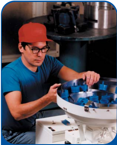
This bowl tooler makes a final adjustment to a vibratory parts feeder, built to singulate and feed caps to a gravity track.
