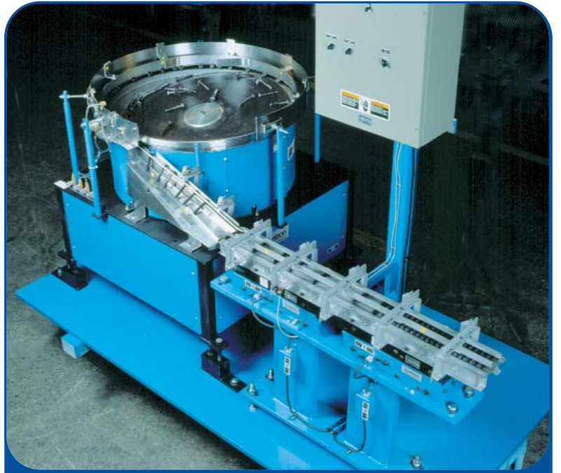
A Syntron® ROF feeder and linear drives form an integrated parts handling system.
